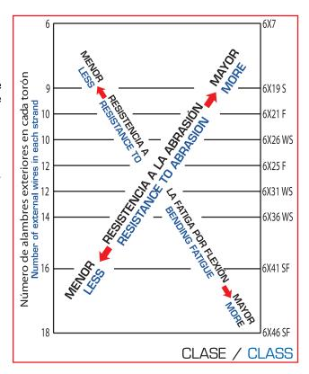
You should also keep in mind that there is a balance between wear resistance and bending fatigue. If you select a wire rope with fatique resistance it is inherent to this selection the reduction in wear resistance. The next table shows this relationship.
